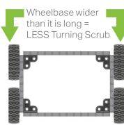
2. Use different wheel and/or tire types to reduce the friction of Turning Scrub:
