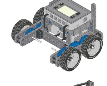
Option 2: Follow the assembly instructions to complete and test the Standard Drive Base then continue using the assembly instructions to build and complete the claw, tower, and object holder. Suggested test objects to use for full Clawbot IQ testing are VEX IQ Challenge game objects, tennis balls, cubes, or any similar object.
