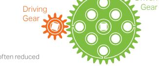
**Note:** Gear Reduction is seen as a fraction that is often reduced to simplify the expression Driven Gear.
