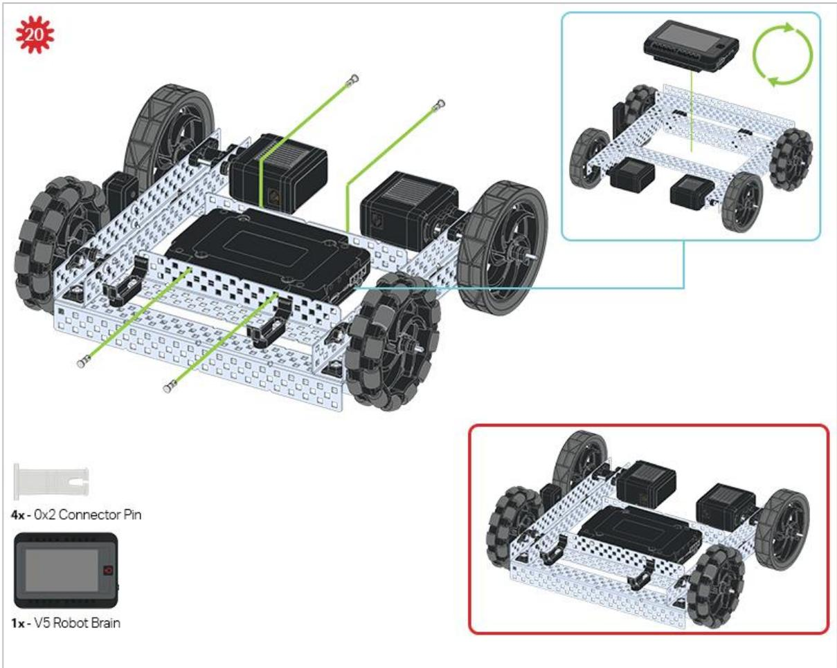
*The blue call out shows what the orientation of the Robot Brain should be if the build were flipped right side up. Make sure the 3 wire ports on the Robot Brain are facing the V5 Radio!*
