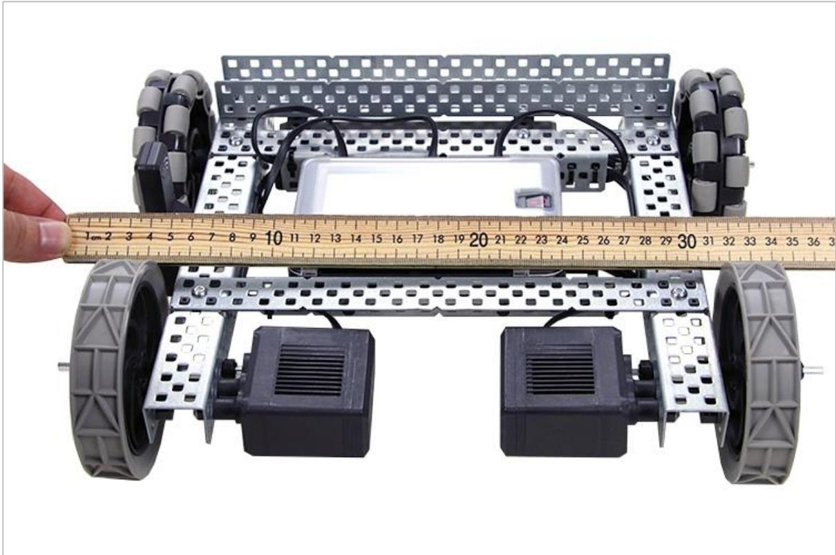
*Measuring the width of the VEX V5 Speedbot*
