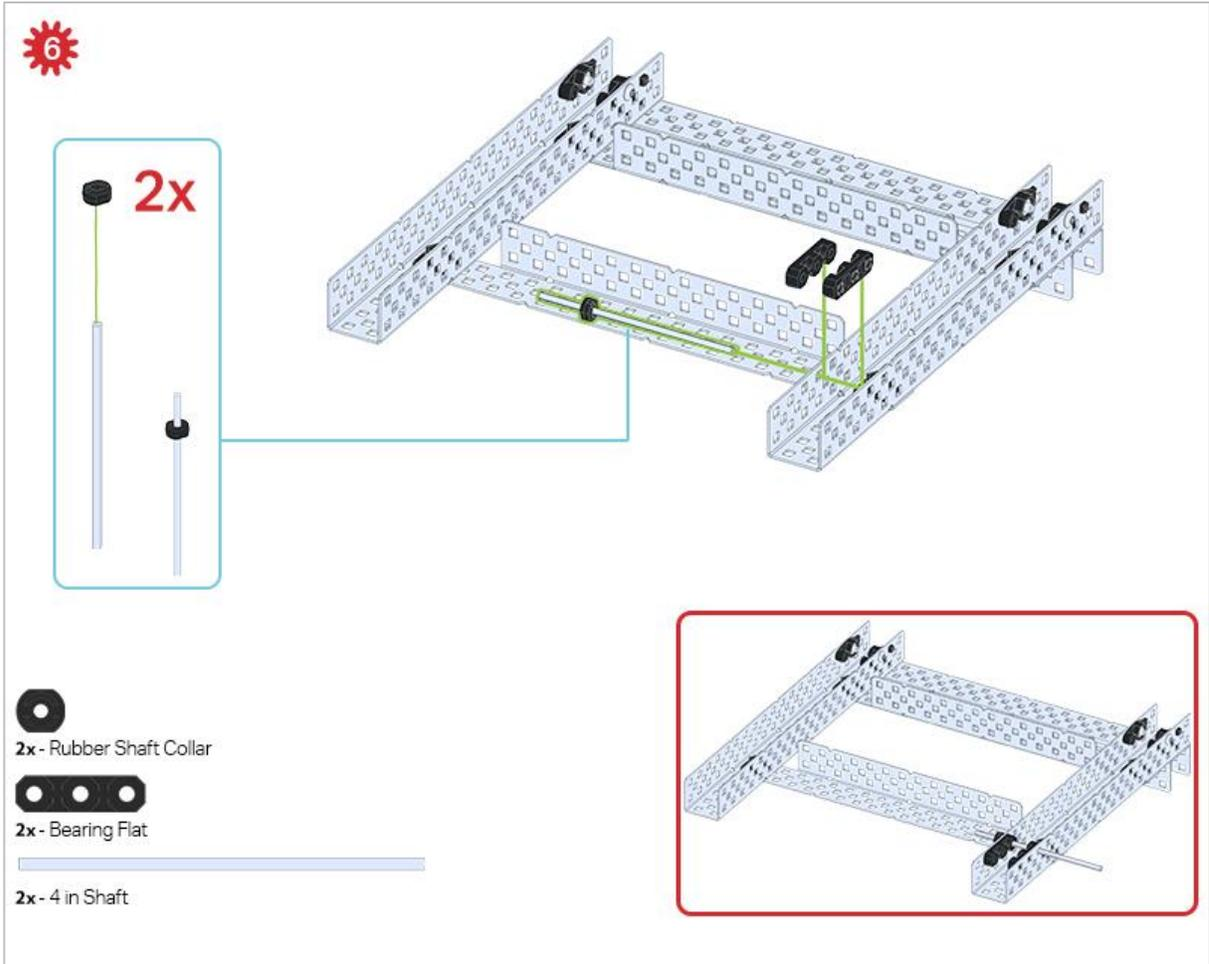
*Only one of the two sub-assemblies made in this step is used right now. The other will be used later in step 9.*
