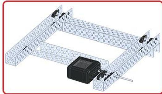
*Make sure your Smart Motors are oriented in the correct direction (screw holes facing the outside of the build and the shaft hole towards the inside).*
