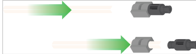
Removal of a standoff from a Mini Standoff Connector
