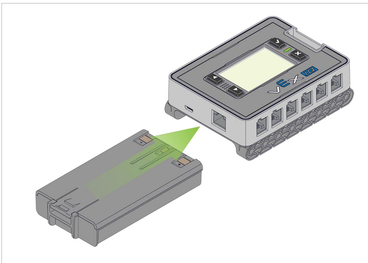
The Robot Battery is inserted into the Robot Brain
