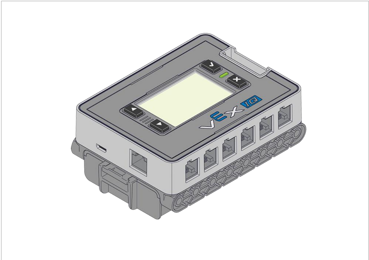
The Robot Battery is securely placed into the Robot Brain
